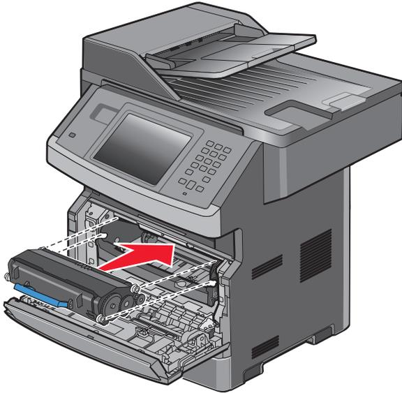
Insert the photoconductor kit and toner cartridge.
