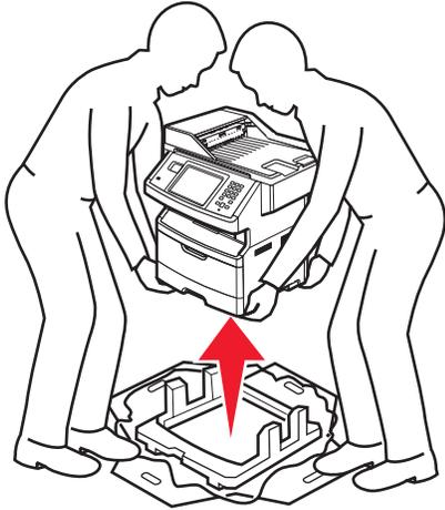
Remove the printer and other components from the box.
