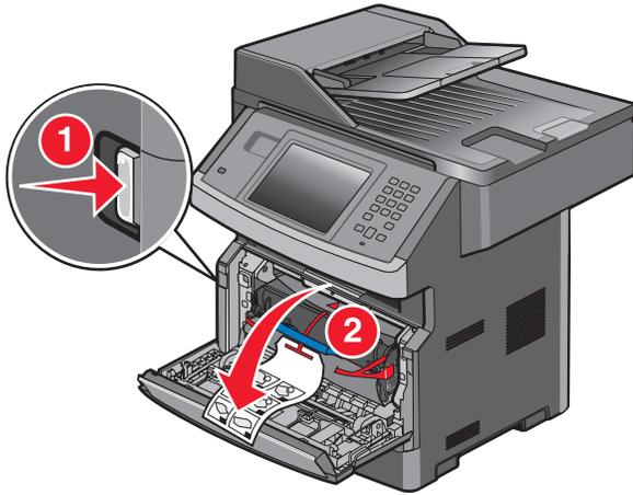
Press the door release button and lower the front door.
