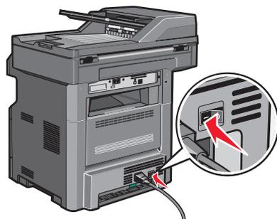
Connect the power cord to the printer and then to a properly grounded outlet that is near the printer and easily accessible. Turn the printer on.
