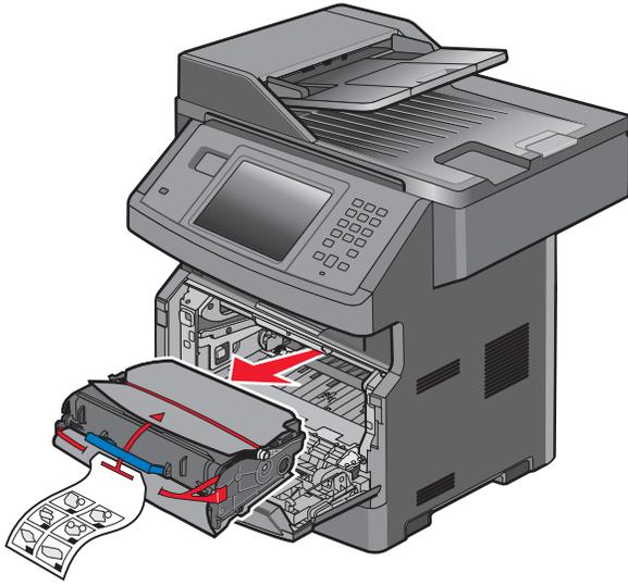
Remove the photoconductor kit and toner cartridge.
