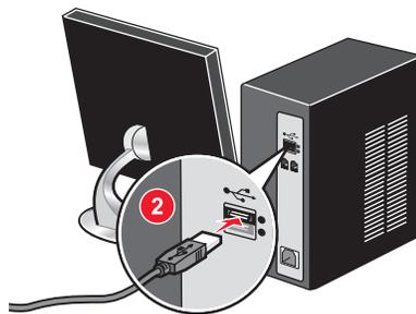
Remove the yellow label covering the USB port. Connect the USB cable to the printer and the computer.
