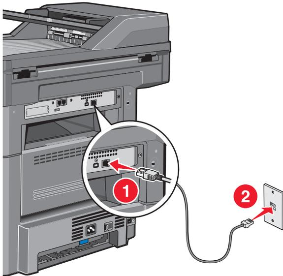
Connect the network cable to the printer and then to the network.
