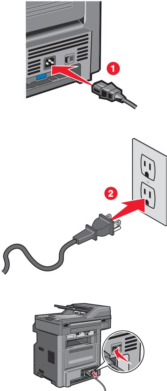
Connect the power cord to the printer and then to a properly grounded outlet that is near the printer and easily accessible. Turn the printer on.
